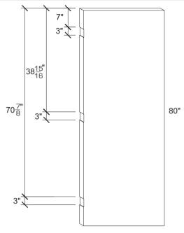
The location of the hinges varies according to the height. Take measurements from the top of the door.
